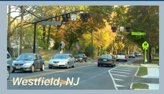
Pedestrian Activated HAWK Signal (High-Intensity Activated crossWalk beacon)
