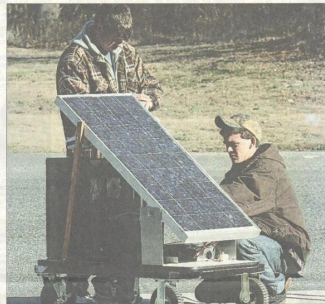
Cape May Technical School students Donny Long, 18, of Wildwood Crest, left, and Elijah Gandy, 17, of Corbin City, work on a solar powered tailgating device for their environmental engineering class. The unit charges a battery that can power a small refrigerator and electric grill.
